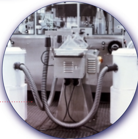
Spot suction on compressing and dust extraction equipment in the pharmaceutical industry.
